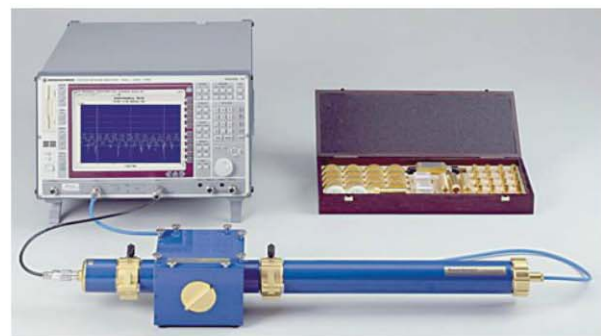
Fig. 3 — Measuring of transfer impedance and screening attenuation of connectors and assemblies with Triaxial Cell and tube-in-tube according to IEC 62153-4-7 .
